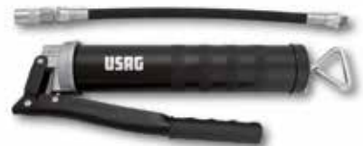
421 Lever operated grease pumps - Model with automatic grease feed to be filled from a bulk container or from a cartridge - Feed pressure 400 bar - Supplied with flexible connection 300 mm and four-claw gripping tweezers - Threaded connection M10x1 - Sheet steel body
